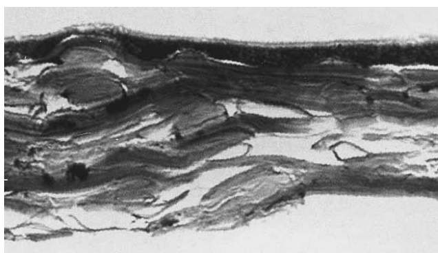
13. Low coating weight cross section at 18 g/m²
