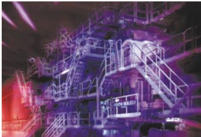
The forming section of a modern paper machine, in this case a Voith Sulzer gap former, designed to produce woodfree coated paper at 1500 m/min
