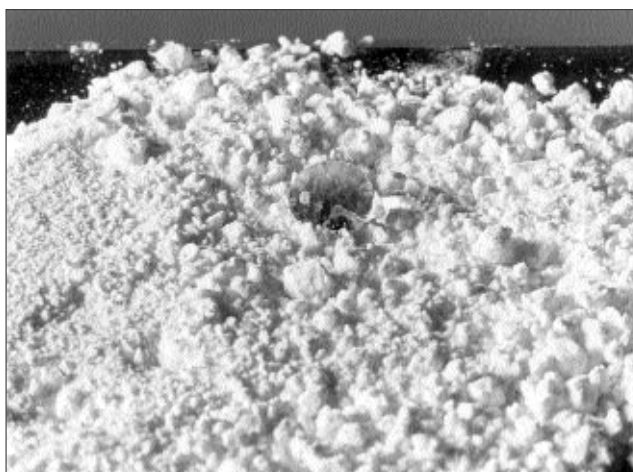
2. A drop of water applied to a powdered sample of the calcium salt of ASA—the high contact angle indicates that the ASA salt is hydrophobic
