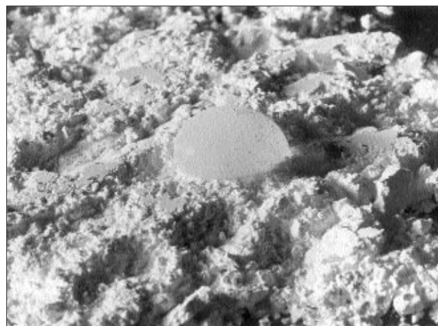
3. A drop of water applied to a precipitated calcium carbonate treated with 1 kg/ton of hydrolyzed ASA—the high contact angle indicates that the calcium carbonate surface is hydrophobic
