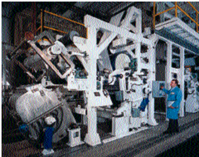
A close-up of the airknife and inverted blade coating stations.
