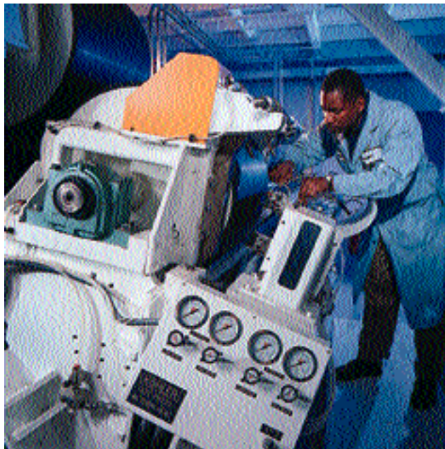
The metered size press is gaining in popularity in North America for efficiently coating lightweight, newsprint, web offset, specialty papers and paperboards.
