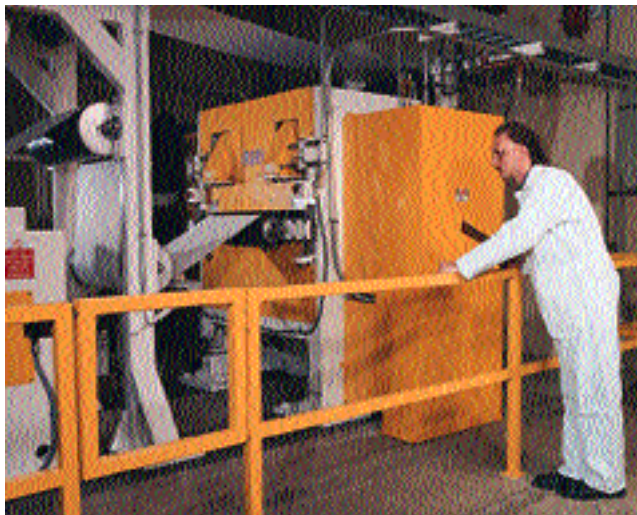
The hot soft nip calender is located on-line for metered size press and other specialized finishing applications.
