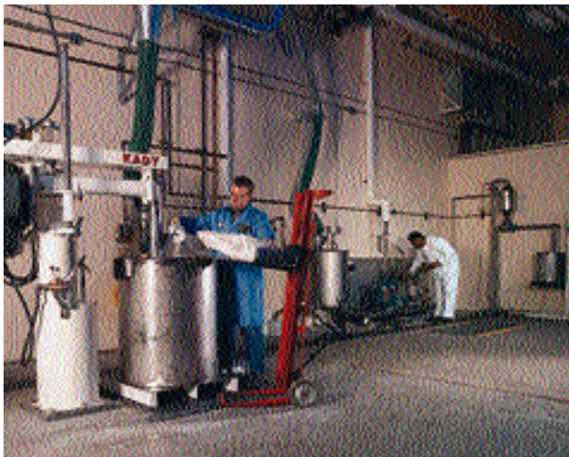
The coating kitchen, located just a few feet from GenCorp Specialty Polymers' new high speed pilot paper and paper-board coater, is capable of preparing a wide range of pigmented and starch formulations.
