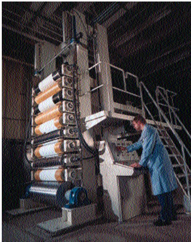
The pilot coater supercalender finishes and prepares rolls for customer print trials.
