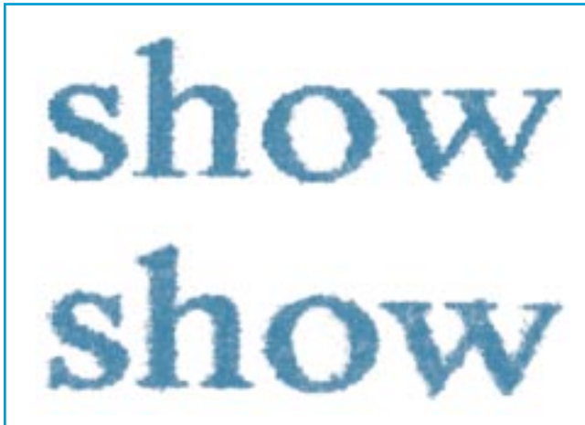
5. Image analysis of text for two ink-jet prints with a threshold of 190. Sample A: area = 9.68 mm 2 , perimeter = 65.6 mm, OD = 0.82. Sample B: area = 10.82 mm 2 , perimeter = 68.8 mm, OD = 0.77.
