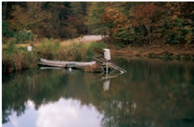
Pond monitoring probes are in the center of this photograph. The intake and outflow lines are the two pipes running diagonally into the water.
