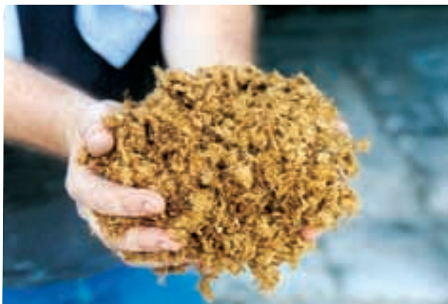
This press cake typically has 50% solids and has excellent combustion characteristics.
