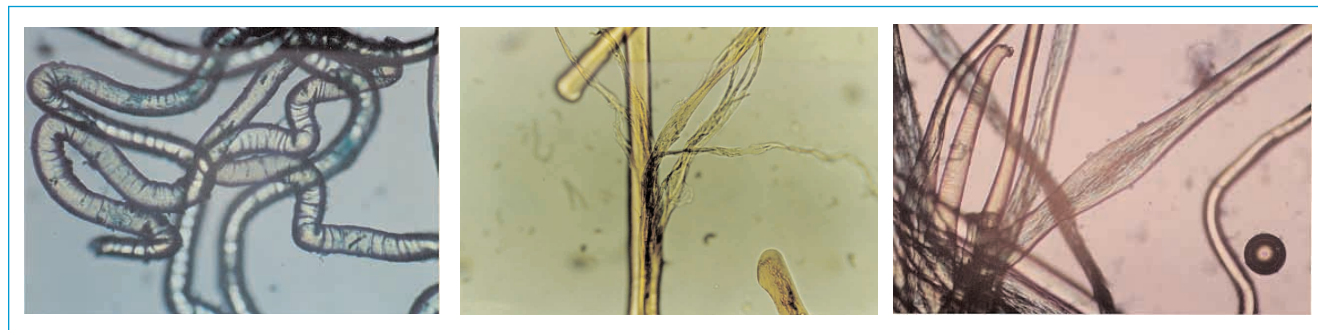
2. Microscopic analysis. Left, fiber damaged chemically; center, damage from an external mechanical source; right, damage from an internal mechanical source.
