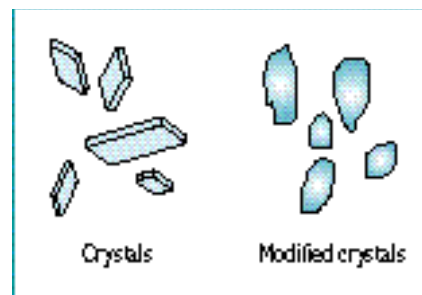
5. Addition of a modifier alters crystal habit, which prevents formation of hard, dense deposits
