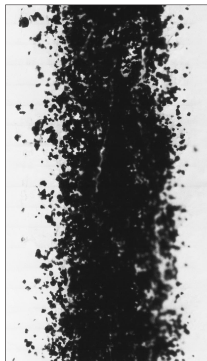
7. Microscopic photograph (40 \times ) of swelling-induced cracks in a line of toner. (The toner line is oriented along the machine direction of the paper; cracks occur preferentially along the cross-machine direction of the paper.)
