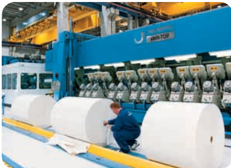
Roll wrapping through labeling is totally automated.
