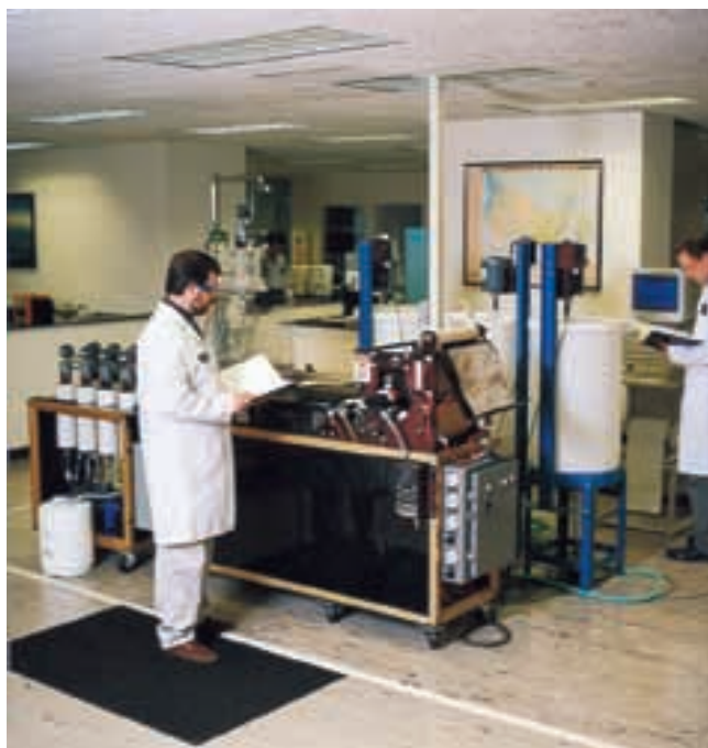
Glover prepares M/K Sheetformer for operation.
