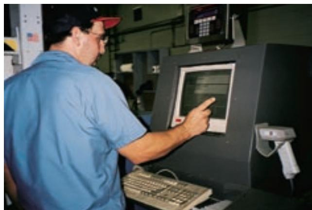
5. An operator selects a work order number to be converted by using a touch-screen monitor.
