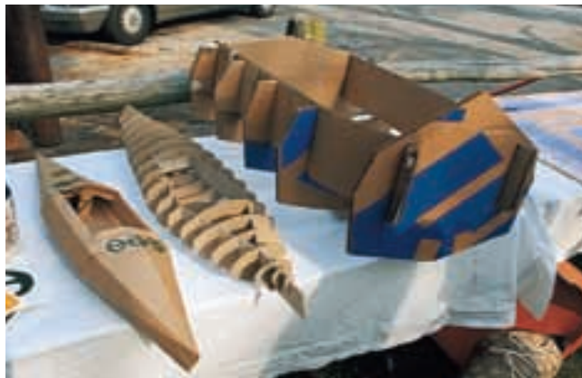
Models of the internal structure (above) demonstrated the design work that went into building the full-scale kayak (below).
