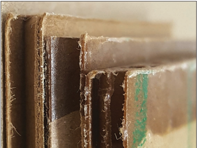
3. Three specimens from the same material cut with cutter 5. The left side of each specimen was face up in the cutter, and the blade impinged first on the leftmost surface. Note that both liners are curled in the same direction because of the force of the blade pressing down during cutting. The left specimen is unwaxed and appears as cut. The middle specimen is after edge waxing. The rightmost specimen has been tested, with a clear edge bias following the initial edge curl. Specimens were identically sized and are offset one from another in the image for visual clarity. Few samples have this dramatic an edge curl, but many samples cut with the various cutters have some observable edge impact.
