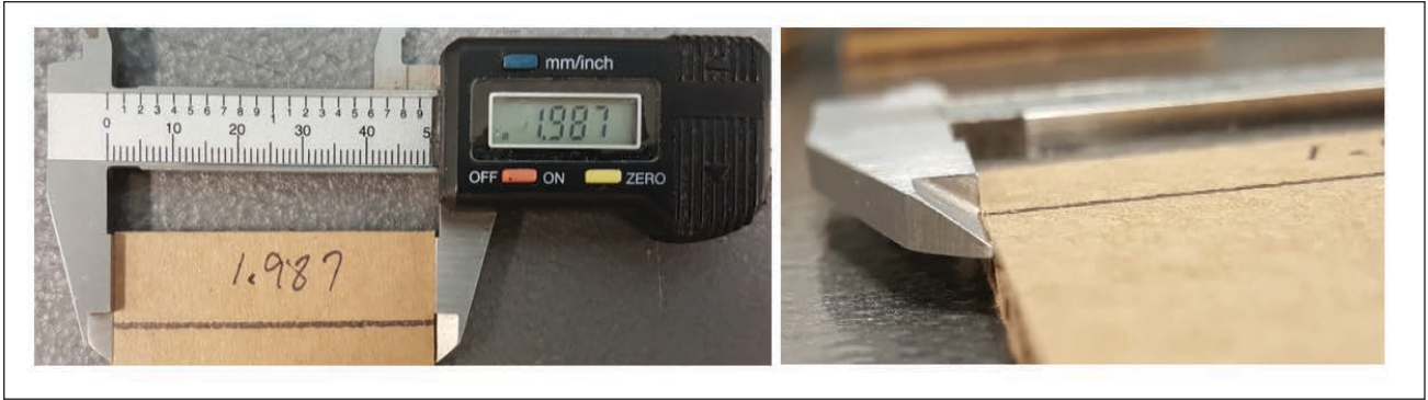
1. Images of the measurement of a sample specimen. Note that the jaws of the caliper, resting on a level surface, are elevated above the surface and so measure just the area of the upper facing at one edge.
